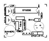
Circuitboard here, in natural size, measures: 29x38mm. On the circuitboard you will find, alarm summer, potentiometers, lightsensor and wire connectors.
